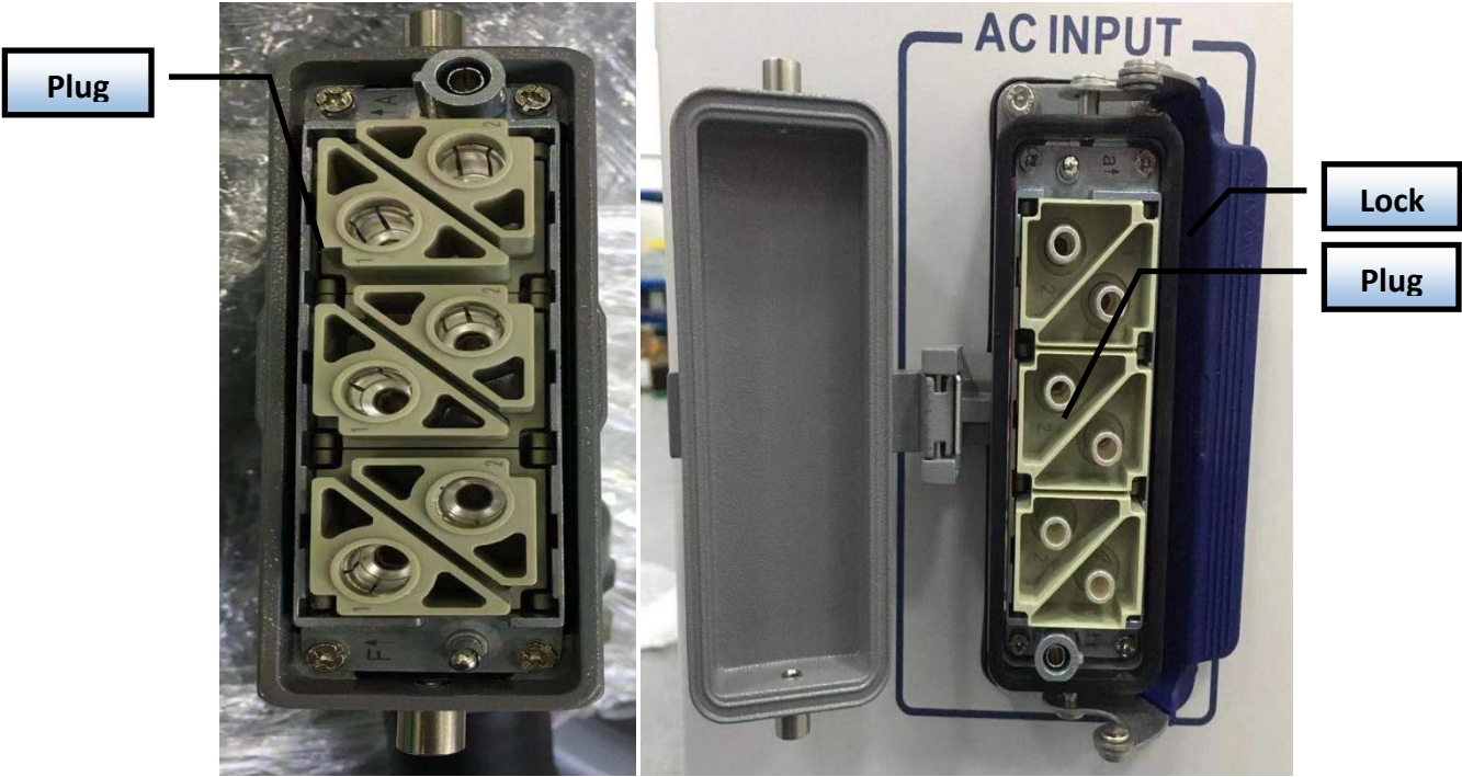
Figure 8 RFL-C20000XZ physical picture of power cord plug and socket
