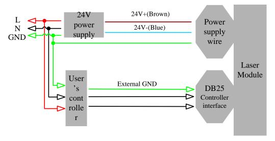
Figure 4. Schematic of recommended electrical connection
