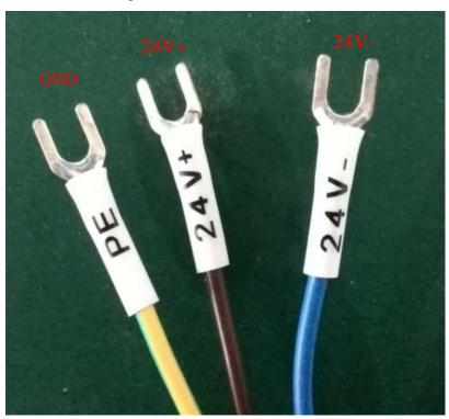
Figure 3. Definition of power line wires
