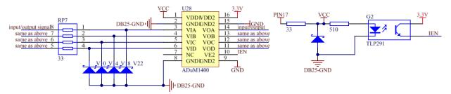
Figure 6. Schematic of input and output signals.
