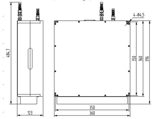
Figure 1. Dimension drawing of laser module (Unit: mm).
